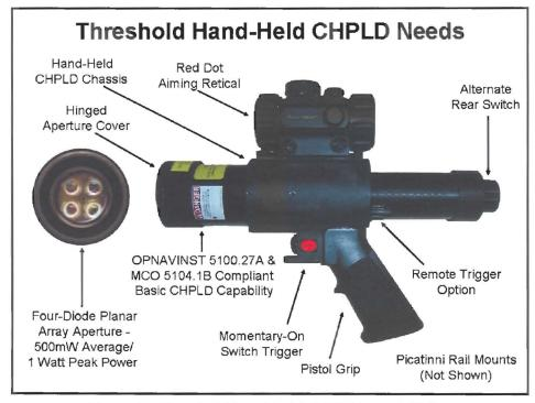
Figure 7. Threshold hand-held CHPLD capabilities.
