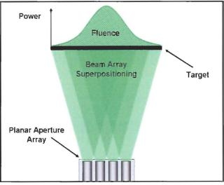
Figure 2. CHPLD laser beam geometry.
