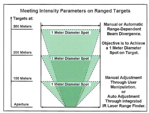
Figure 6. Continuous CHPLD spot diameter adjustment for maintenance of constant fluence.
