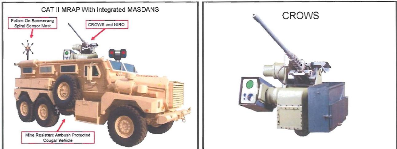
Figure 8. CROWS-armed MASDANS capability. Figure 9. CHPLD integrated with the CROWS.
