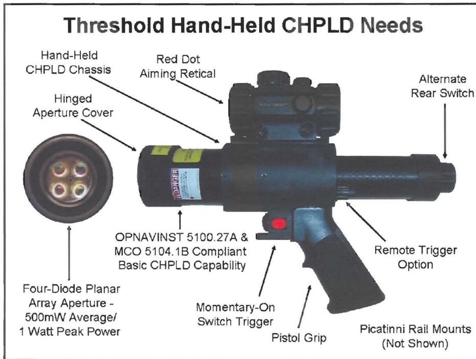
Figure 7. Threshold hand-held CHPLD capabilities.
